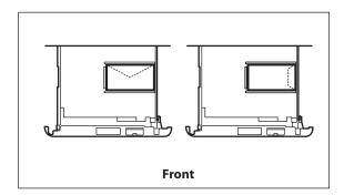
Align the leading edges of the envelopes, and make sure that they are held in place under the claw.
