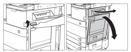
2 Remove any jammed paper protruding from the inside slot of the copy tray.
