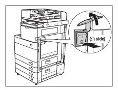
Wait at least 10 seconds after the Main Power Indicator is turned off, and then turn the main power switch back to "I" side.
