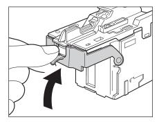
Gently push the staple case back into the finisher until it is securely in place.
