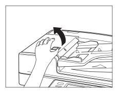
Clean the rollers (a total of three places) inside the feeder cover with a cloth dampened with water. Then, wipe the area with a soft, dry cloth.
