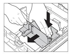
Fix the front width guide in place with the screws.
