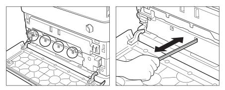
4 When you have finished cleaning the dust proof glass, gently push the dust proof glass cleaner back onto the rear side of the front cover.
