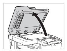
9 Clean the feeder scanning area with a cloth dampened with water. Then, wipe the area with a soft, dry cloth.
