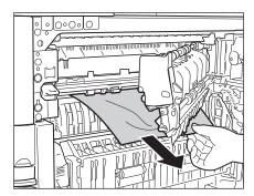
Pull down the inner guide, and remove any jammed paper.
