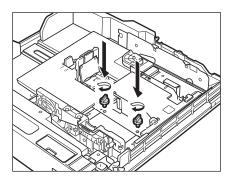
Move the back width guide of the envelope feeder attachment in accordance with steps 6 to 8.
