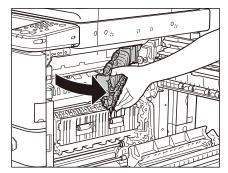
**3** Remove any jammed paper inside the machine.
