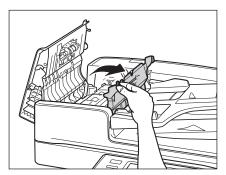
4 Clean the rollers (a total of three places) inside the inner cover with a cloth dampened with water.
