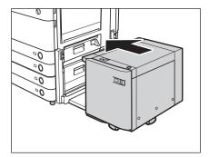
If the screen indicating the paper jam is no longer displayed after reconnecting the paper deck unit to the main unit, proceed to step 7.
