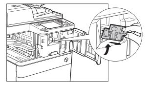
3 Press the area indicated by PUSH, and then lift up the staple cartridge.
