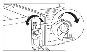
Open the top cover of the puncher unit.
