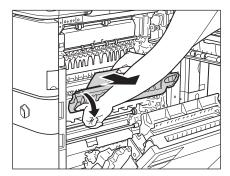
After the jammed paper is removed, return the upper cover of the fixing unit back to its original position.
