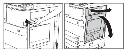
Remove any jammed paper in the upper part of the duplexing unit.
