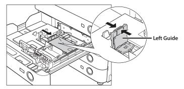
Gently push the paper drawer back into the machine until it clicks into place in the closed position.
