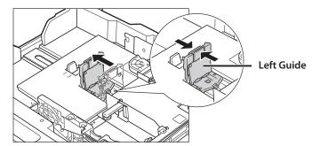
4 Load 10 envelopes at a time with the side you want to print on facing up. While loading the envelopes, press down on the left side of the receptacle to lock them into place.
