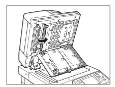
Clean the feed scanning area with a cloth dampened in water or a mild detergent, and then wipe the area with a soft dry cloth.
