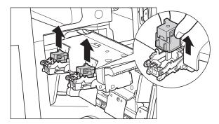
On the staple case, push down Part A to unlock, and then push up Part B.
