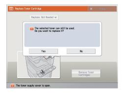
4 Wait for the internal cover to open automatically, and pull the toner cartridge out of the toner supply port.
