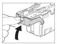
6 Gently push the staple case back into the stapler unit until it is securely in place.
