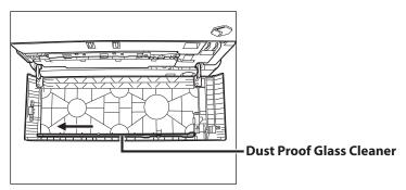
Hold the dust proof glass cleaner so that the pad on the tip is facing down, push it back as far as it goes, and then slowly move it up and down.
