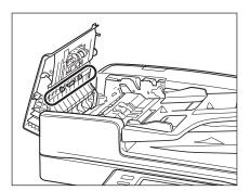
Open the inner cover, holding it by its front tab.
