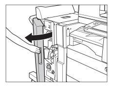
2 Tilt the upper delivery guide to the right, and remove any jammed paper.
