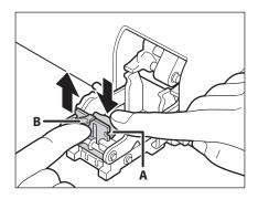
Remove any jammed staples, and return Part B to its original position.
