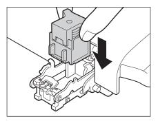
Pull the stapler unit of the saddle stitcher unit towards you, and then push it down into its original position.
