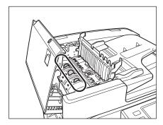
5 Clean the transparent plastic part of the inner cover with a cloth dampened with water. Then, wipe the area with a soft, dry cloth.
