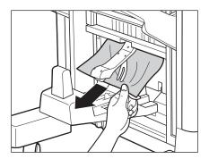
Tilt the lower delivery guide to the right, and remove any jammed paper.
