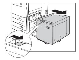
2 Pull down the green lever on the side of the paper deck that attaches to the main unit, and remove any jammed paper from the feeding area.
