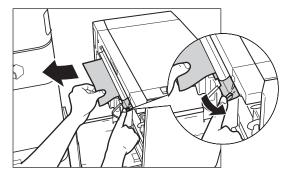
Paper can also be jammed in the feeding slot on the side of the main unit. Remove any jammed paper from the feeding slot.
