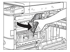
Remove any jammed paper inside the machine.
