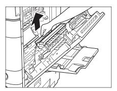
Remove any jammed paper located between the main unit and the lower right cover.
