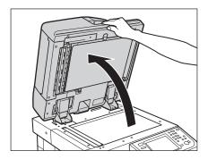
2 Pull the lever above the feeder, and open the document scan cover.
