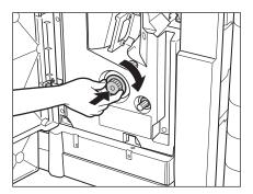
Remove any jammed paper protruding from the output part.
