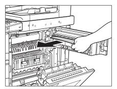
Remove any jammed paper in the lower part of the duplexing unit.
