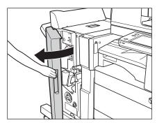
2 Grip the saddle stitcher unit by its handle, and pull it out of the finisher until it stops.
