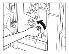
While pushing in the knob on the left, turn it in the direction of the arrow (clockwise).
