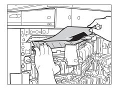
Remove any jammed paper protruding from the output tray.
