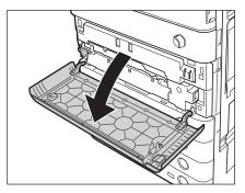
2 Remove the dust proof glass cleaner from the rear side of the front cover by sliding it to the left side.
