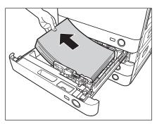
2 Slide the left guide to align it with the mark for the desired paper size.
