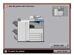
After you have removed all of the jammed paper in the locations indicated on the touch panel display, restore all levers and covers to their original positions.
